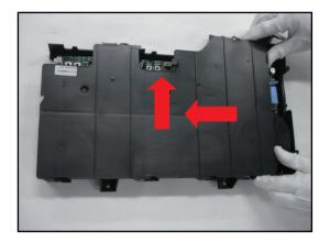
2. Loose two screws on the side of IH module as below.
